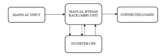
2. Under maintenance operation, the Mains AC Input flows through the MBP unit to the connected Loads – the UPS is not in the circuit.
